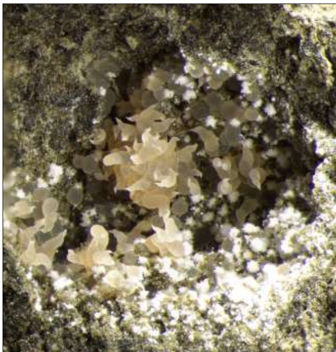
An 8mm cavity with grey to cream lustrous thomsonite spheres and worm-like growths with fibrous thomsonite (white).
